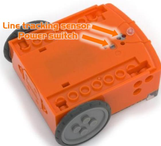
Edison's power switch and line tracking sensor
