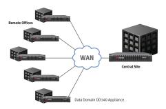
The DD140 comes equipped with EMC Data Domain Replicator software, which provides network-efficient replication so remote office data can be sent offsite over existing networks for centralized management or for disaster recovery. Tape backups can be eliminated at remote offices, reducing costs and simplifying data protection.
